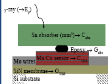
Detector cross section
